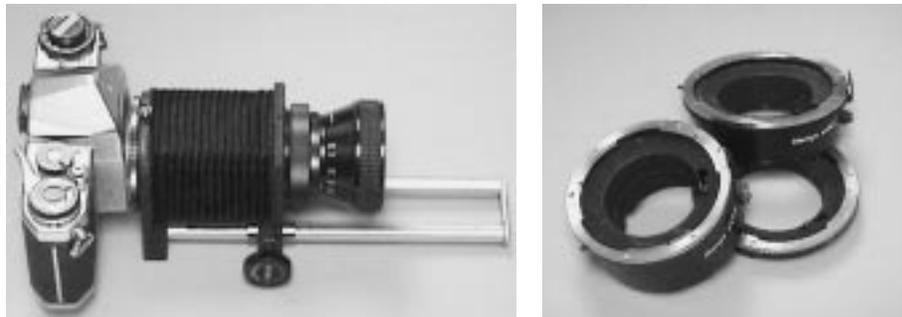
*Figure 1: Bellows (left) and extension tubes (right) provide cameras an ability to image objects larger than life size on film. The greater the distance between lens and camera the closer focusing distances are possible.*
