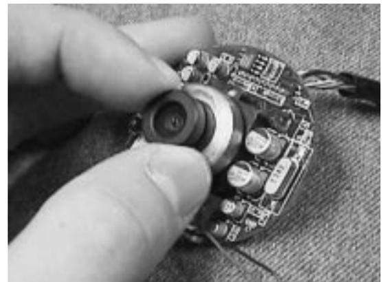
*Figure 3: The Quickcam is an example of a fixed focus digital camera (left). It is possible to change the fixed focus point but the camera needs to be disassembled in order to accomplish this, as is demonstrated on the right.*
