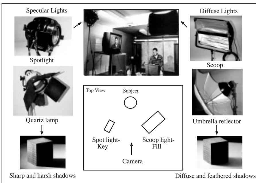
Figure 11: The key light defines the direction, shape and quality of the shadow. The fill light is dimmer, often more diffuse than the key and fills in the shadow cast by the key. The fill light intensity can be adjusted by moving the light back forth or adjustment of a light attenuator such as barn doors.
