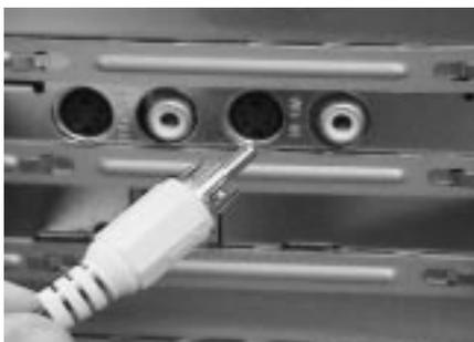
*Figure 6: These are the video input/output ports of a video capture card on the back of a computer. A video capture or digitizing card takes input from a standard analog video source and converts it to digital data.*
