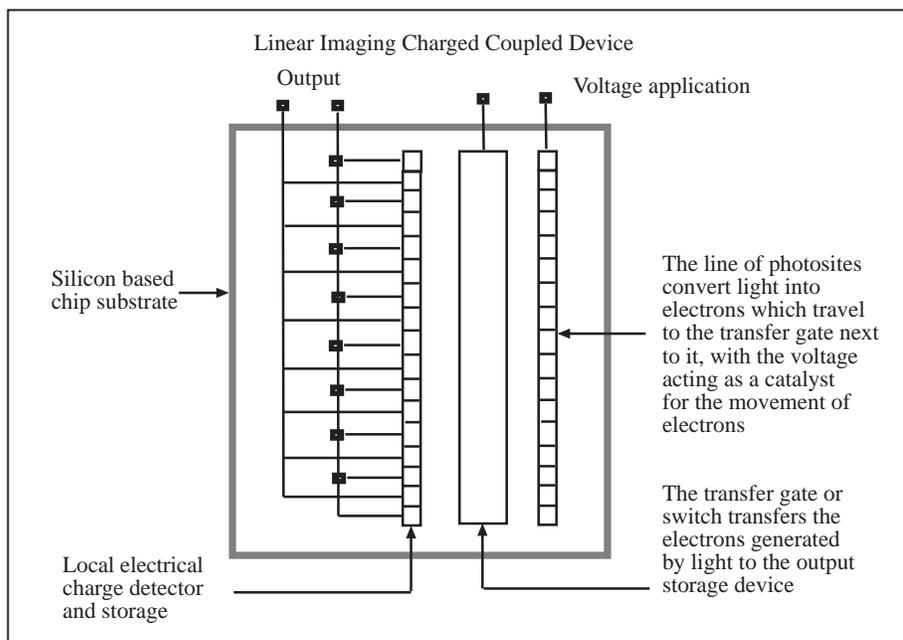
*Figure 7: The basic structure and operation of a CCD or charged coupled device.*
